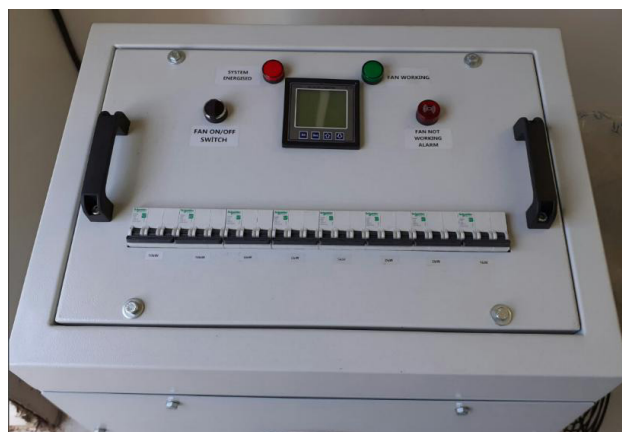
Load Bank / Dummy Load
